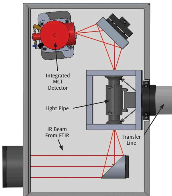
Optical geometry of the GC-FTIR Accessory.
