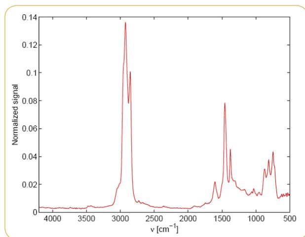
Heavy oil spectrum collected using the PAS301 (8 cm<sup>3</sup>, scan time 25 s)
