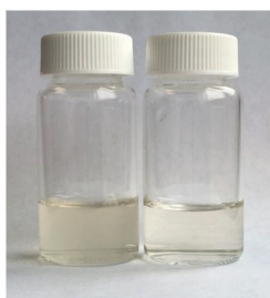
Figure 1. Sample: whole blood following zinc sulfate precipitation and centrifugation. Left vial unfiltered; right vial filtered using ISOLUTE® FILTER+ plate.
