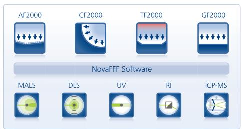
The flexibility of the Postnova FFF Platform is manifested by the fact that all mayor modules can be used at the same time for Flow FFF, Centrifugal FFF and Thermal FFF. Many modules, such as the pumps, degassers, auto injectors, fraction collectors and detectors can be shared between the FFF technologies. All is controlled by the single NovaFFF software and also detectors such as MALS, VISCO, DLS and ICP-MS are integrated making data analysis and evaluation a simple task.
