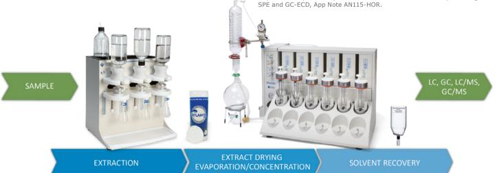
Workflow for the Boptage\* Horizon 5000 Extractor, used with Atlantic\* solid phase extraction disks, the DryVap\* In-line drying and concentration system and the Biotage\* SolventRecovery SVOC for a full sample preparation system.
