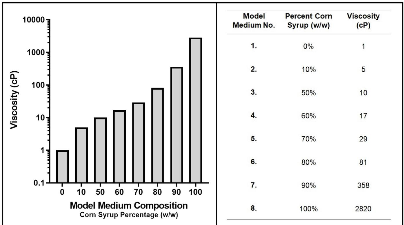
Figure 1: Overview of the model medium strategy using during the magnetic decoupling characterization. Viscosity range was determined based on reported values from biopharmaceutical, agricultural, and industrial upstream processes.
