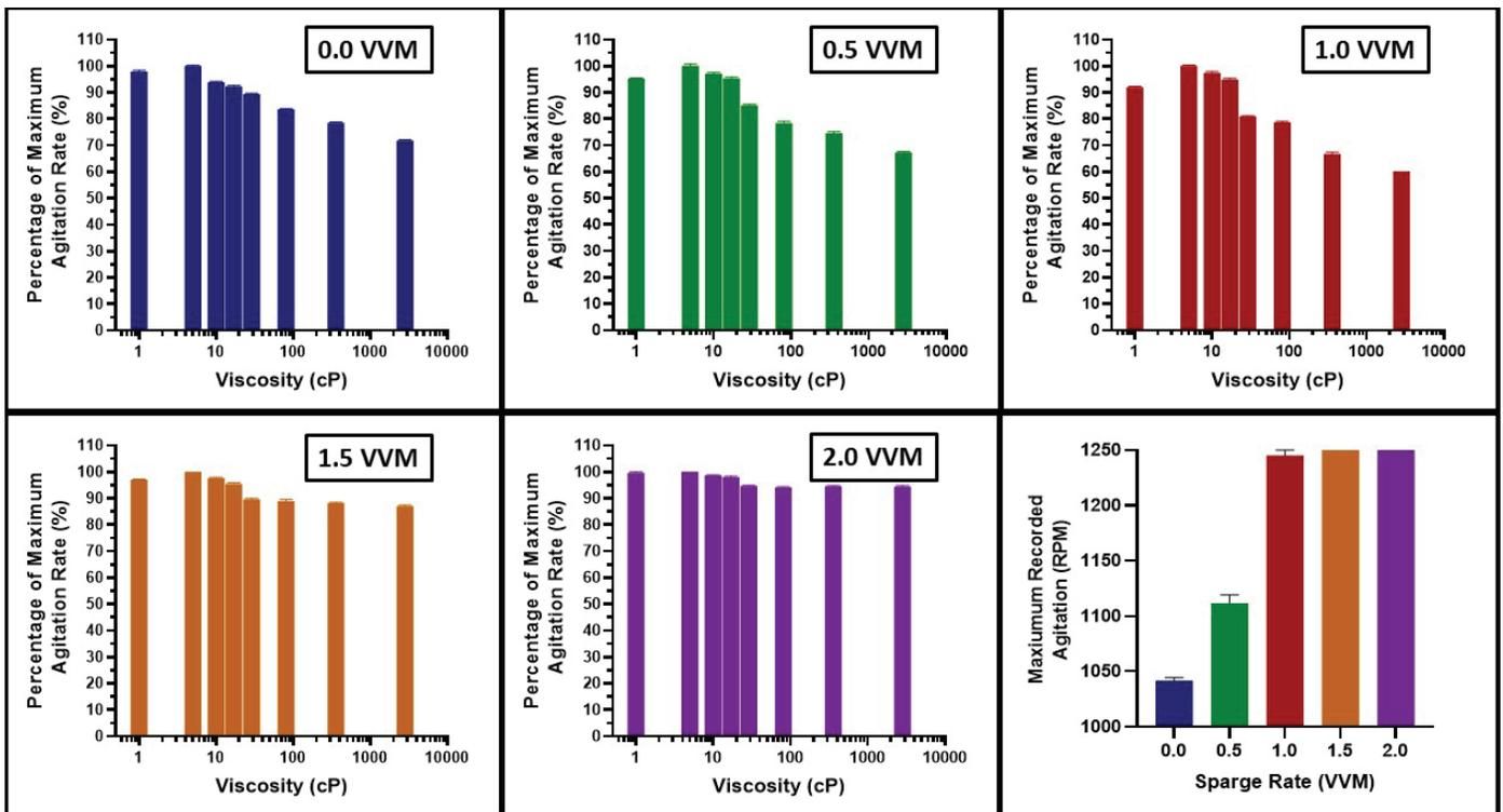
**Figure 3: Normalized viscosity testing data across different aeration strategies.** Results demonstrate that sparged air flow rates of 1.5 and 2.0 vvm can effectively mitigate some of the effects of higher media viscosities to support higher agitation rates in magnetically coupled agitation systems.
