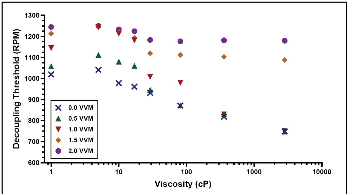
**Figure 2: Results of magnetic decoupling characterization study.** Results demonstrate that magnetic decoupling agitation rate threshold decreases with an increase in system media viscosity. Data also show how increases bottom air aeration rate can potentially mitigate the effects of high viscosity media and increase the magnetic decoupling agitation threshold of the system.
